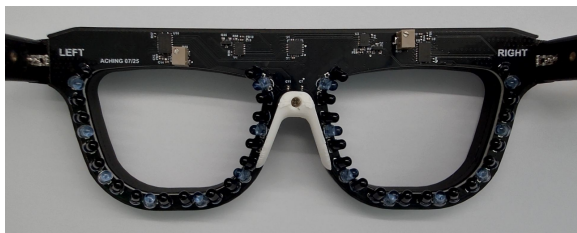
Figure 5: The gaze tracking daughtercard. It contains a pattern of sixteen LEDs and eight phototransistors per eye, allowing us to sense changes in eye position.
